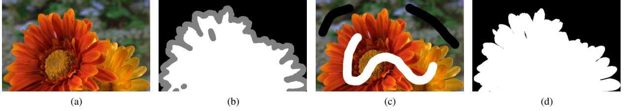
Fig. 1: The matting process: (a) An image to perform matting on, (b) User supplied trimap where black indicates known background, grey the unknown region and white the known foreground, (c) the Scribble alternative to a trimap with white for known foreground and black for known background, and (d) a resulting alpha matte after matting is performed.
